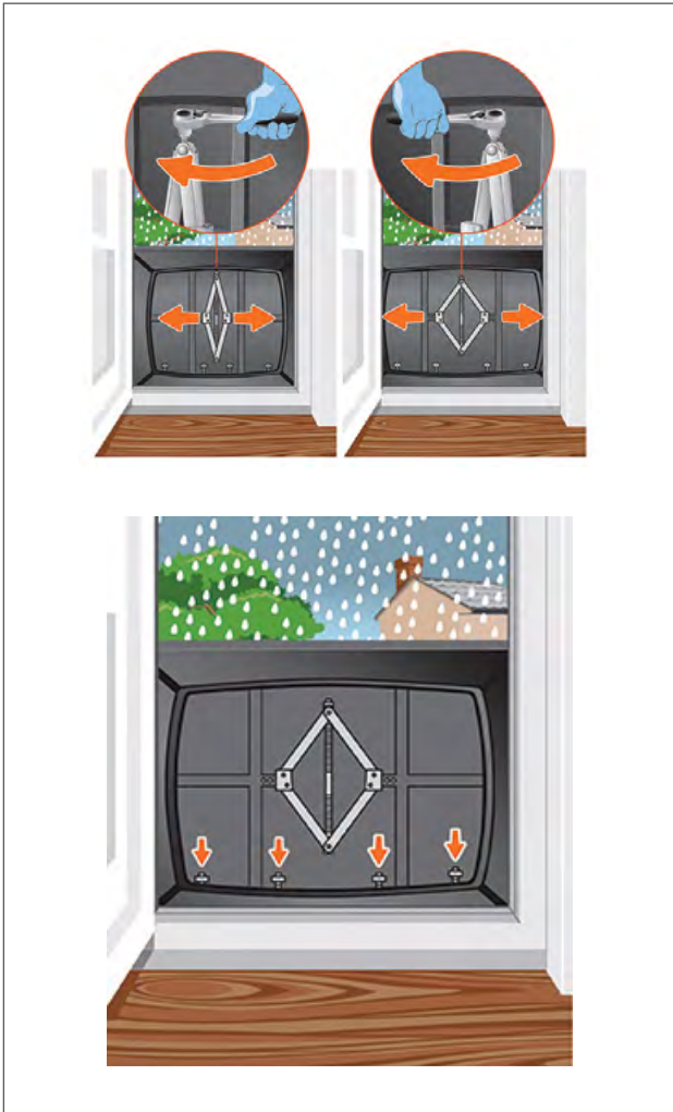
The Floodgate barrier is placed between the doorway and the jack is expanded by using a ratchet wrench, to lock in the barrier horizontally (images on top). The wrench is then used to tighten the four bolts at the bottom, to lock in the barrier vertically (image below). After the flood has receded, the four bolts at the bottom are loosened and the jack is compressed to remove the Floodgate barrier from the doorway. Images: Floodgate Limited.
